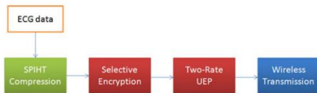
Figure 4 Secure and energy efficient ECG transmission scheme
